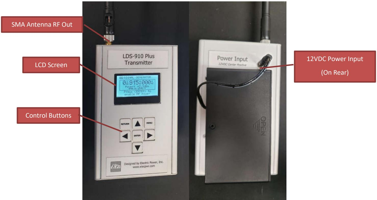
Figure 3 – Transmitter Layout
