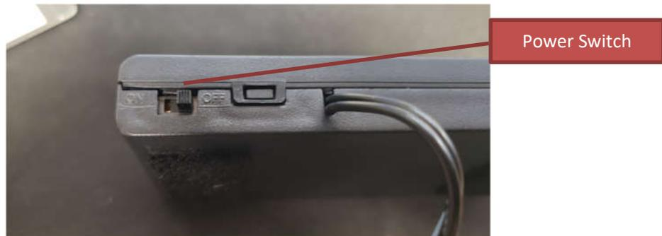
Figure 4 – Transmitter Battery Pack Power Switch Location
