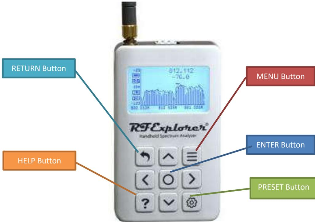
Figure 6 – Receiver Button Layout
